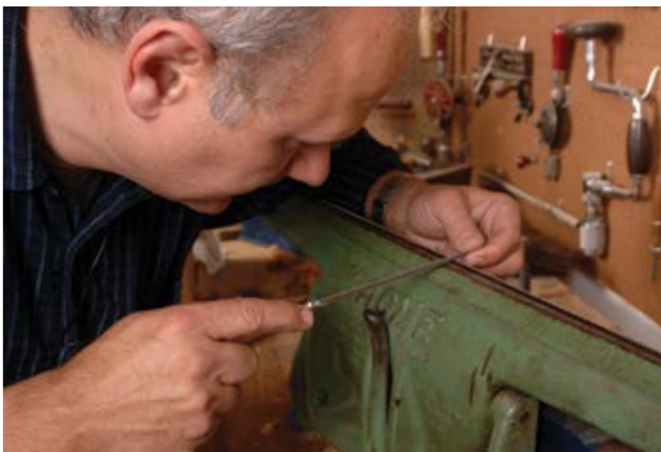
Crouch until you're almost at eye-level with saw teeth, viewing them from side-on
