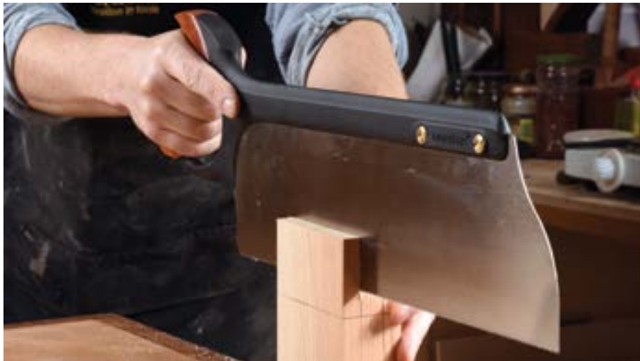
More steel in both directions means deeper and longer cuts
