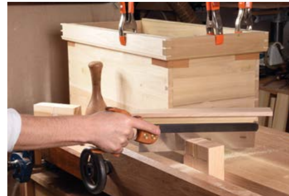
A 018 gauge 300mm long Bad Axe Stiletto dovetail saw can work at full capacity on stock up to 40mm thick
