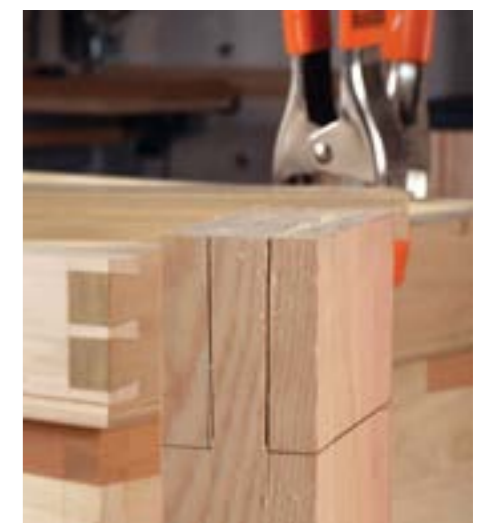
The finer gauge plate on the left has started to distort in the cut and run off
