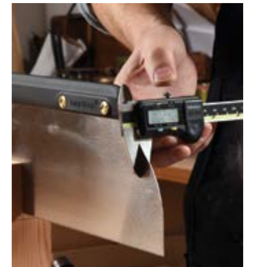
024 is a typical gauge for 410mm long and over tenon saws
