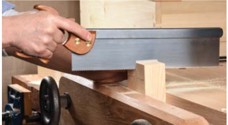
A 020 gauge small tenon, dovetail hybrid saw is well within its working parameters on timber up to 50mm thick
