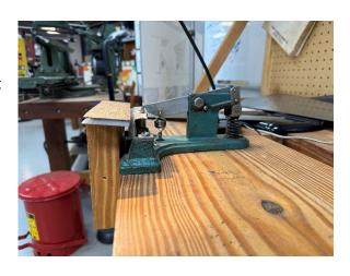
the bevel line to go below the gullet. The idea is to impart a coined line delivered by the beveled anvil just above the gullet. If you striking below the gullet onto the main body of the plate, you will dimple the main body of the plate just above the teeth, which invites cut friction and undermines your set.
