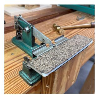
inches off the floor. You'll need to auger a hole to allow the travel rod clearance through the benchtop, and another hole for access to the set strength spring wingnut to adjust tension. Use the underside of the set as a template for hole placement.
