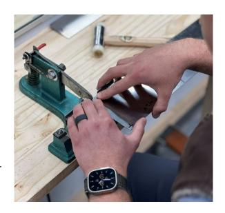
dotted tooth you're going to strike. Resist the tendency to lift the hammer high, because then you cannot see where it will strike center of mass on the tooth. Rest the Hammer on the tooth before striking it and make adjustments to ensure you're going to hit center of mass. Then activate the strike with your foot pressing down on the treadle. You'll get the hang of it as you go.
