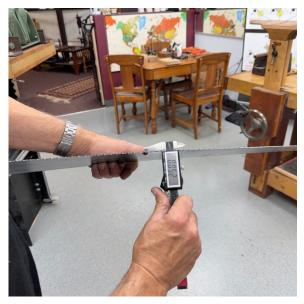
Assessing for accureacy: after striking one or two teeth, examine the tooth on the opposite side of the strike and look for the coined bevel line imparted by the anvil, which should be located just above the gullet. If you're too high or too low, make necessary adjustments to the fence before proceeding. Once you have your bevel line synced to the pitch you're setting, strike about a dozen teeth on both sides of a saw plate. I generally do this at the heel end of the plate before setting the
