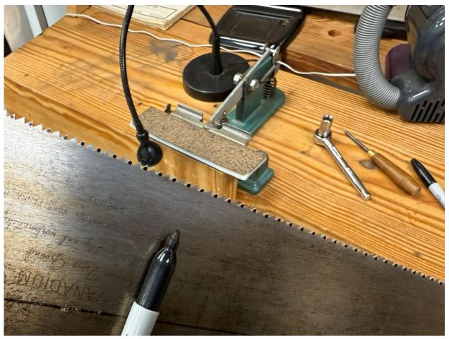
well, or you're lacking in confidence. The idea is to aim small and hit small precisely center of mass on the tooth. Accuracy matters. Obviously, you're going to dot alternating teeth on both sides of the toothline to avoid striking the same tooth in different directions.
