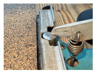
Make a ramp to support the sawplate. Take note in the video how I have built a small ramp surfaced with cork rubber. My crude solution is to cut 8" off a piece of 2 x 6 with my miter saw, such that the top supporting the ramp presents a 5° downward slope toward the anvil of the saw set. This downward slope lessens the acuity of the beveled anvil which otherwise will impart too
